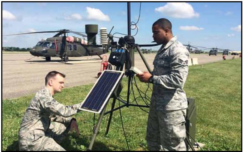
U.S. Air Force Airmen from the 207th Weather Flight, 181st Intelligence Wing, Indiana Air National Guard perform weather observation using the TMQ-53 (tactical meteorological observation system) during a field exercise at Camp Atterbury, Edinburg, Indiana June 5, 2014. The 207th Weather Flight mission was to support 38th ID Aviation assets at Camp Atterbury. (U.S. Air National Guard photo by Lt. Col. Joseph Marcello/Released)
