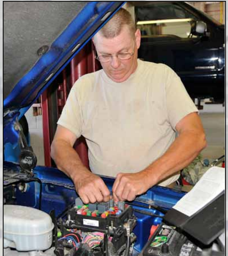
U.S. Air Force Tech. Sgt. Mark A. Ford, 181st Intelligence Wing, Indiana Air National Guard, checks for blown fuses and makes sure relays are working correctly on a Ford F150 truck, Alpena CRTC, Mich., July 16, 2013. (U.S. Air National Guard photo by Senior Master Sgt. John S. Chapman/Released)
