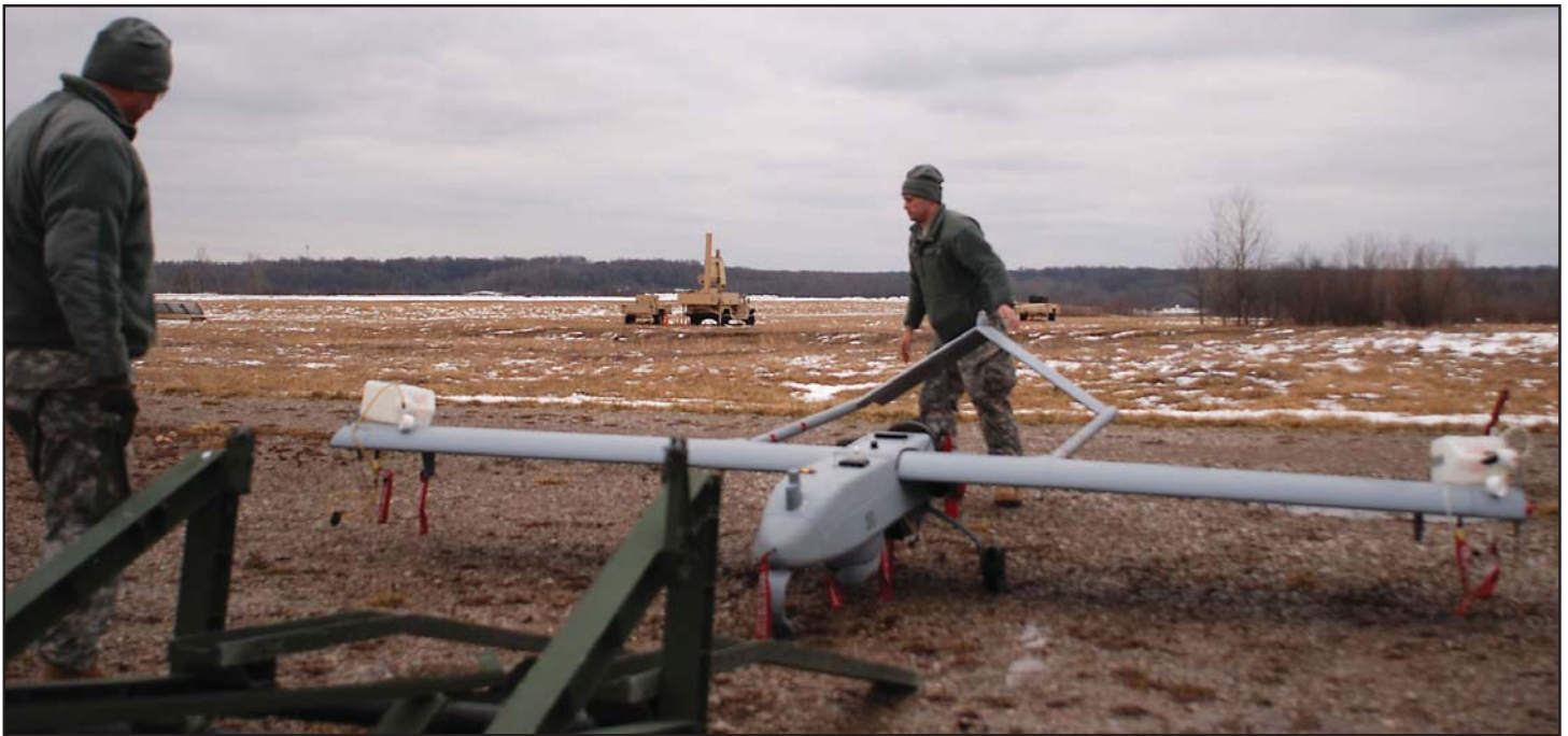
Members of the 76 BSTB prepare to load the RQ-7 Shadow RPA onto the launcher. (U.S. Air National Guard photo by Maj. Frank Howard, 181st IW Executive Staff Officer)
