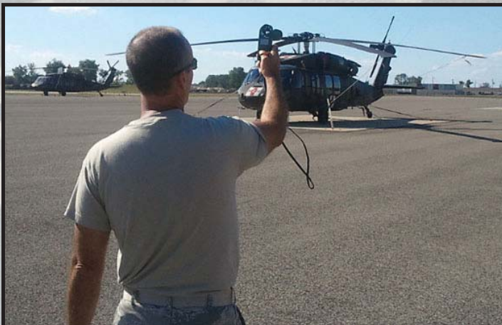
Tech. Sgt. Todd Bock, 207th WF, checks current wind speed, atmospheric pressure, temperature and dew point by using a Kestrel 4500 while at Camp Atterbury back on June 22, 2012. Photo submitted by 207th WF
